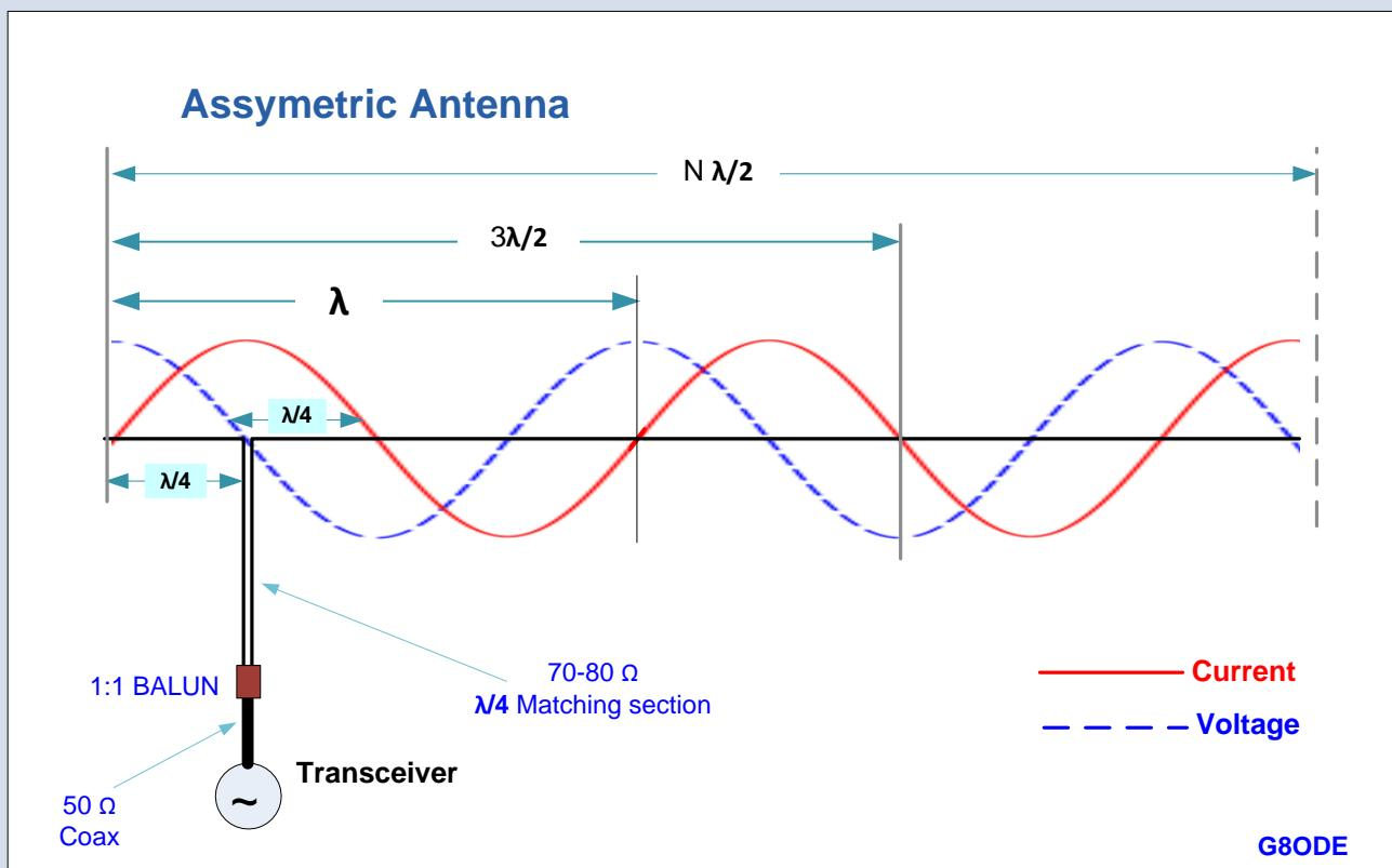
An antenna that is two or more half wavelengths long can be fed with a low impedance transmission line of coax at any of the current maximum positions such as the point a quarter of a wave from one end. In such a case a 70-80 ohms feeder could be used though the impedance is slightly greater than for a half wave dipole. If the antenna is designed for 7 MHz. it will also work on 21MHz , but will be badly matched on the even harmonics on 14 & 28 MHz.
