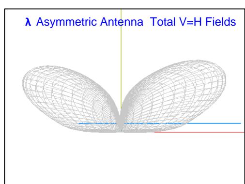
The difference between a one wavelength and one and a half wavelength asymmetrical antenna is fairly obvious when the horizontal far field patterns are observed. The longer antenna has more lobes and improves the DX capabilities of the antenna. The horizontal, fields are very similar with the longer antenna having an additional central lobe.
