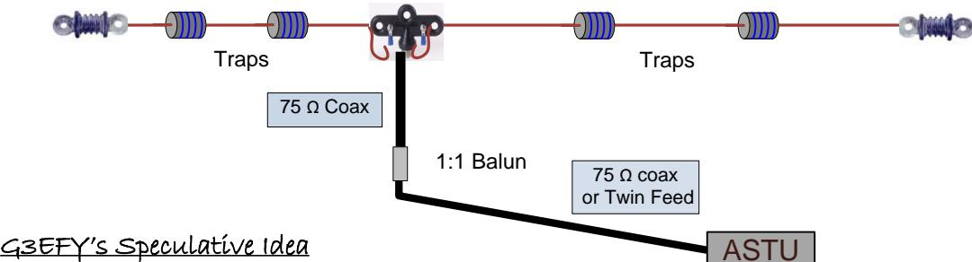
A speculative idea using a trapped version of this antenna, is to replace the usual 50 ohm feeder of a trap dipole with a calculated length of 75 ohm coax with a balun and then a length of 75 ohm twin feed to the ASTU. Thus creating a vertical radiator and possibly increase the DX capabilities of the antenna.
