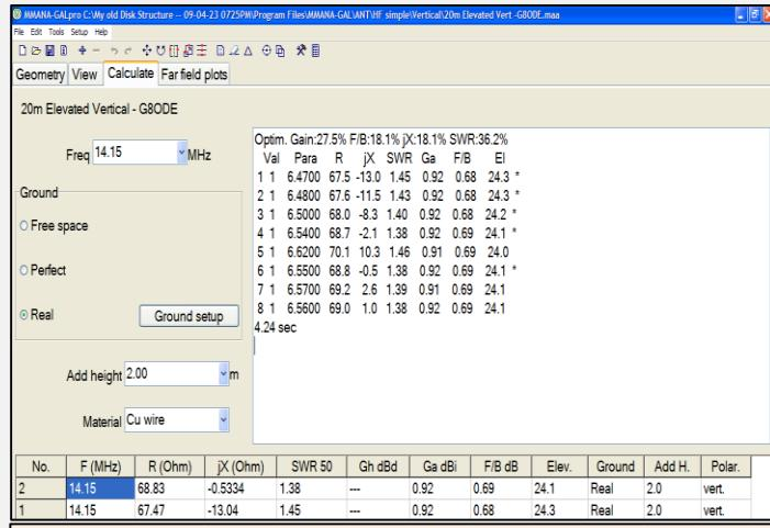
The MMANA-GAL calculations. Line 1 is the first run & line 2 shows the last value recorded after the antenna was optimised for minimum SWR
