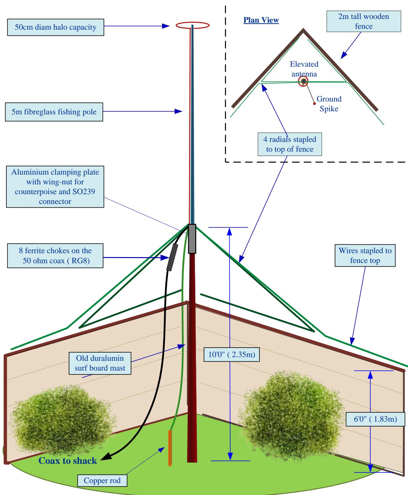
**NOTE:-** The antenna wire is cut to the length calculated by the formula ;
