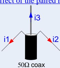
A Ground Plane antenna's radials are provided in pairs and are slightly longer (5-10%) than the radiator. The currents  $i_1$  and  $i_2$  in the radials flow in opposite directions and their fields cancel, consequently only the vertical's current  $i_3$  produces radiation. Ideally the antenna should be at a height of about  $0.2\lambda$  above the ground, if lower then ground losses start to increase unless the ground is good.
