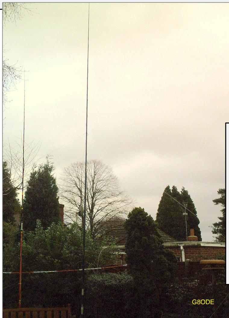
Picture shows the shorter 20m Elevated Vertical “fishing pole” antenna alongside the 40m Vertical.
