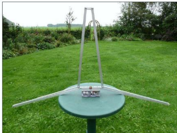
Photos showing how the Foldable Loop is opened up into the operating hexagonal shape.
