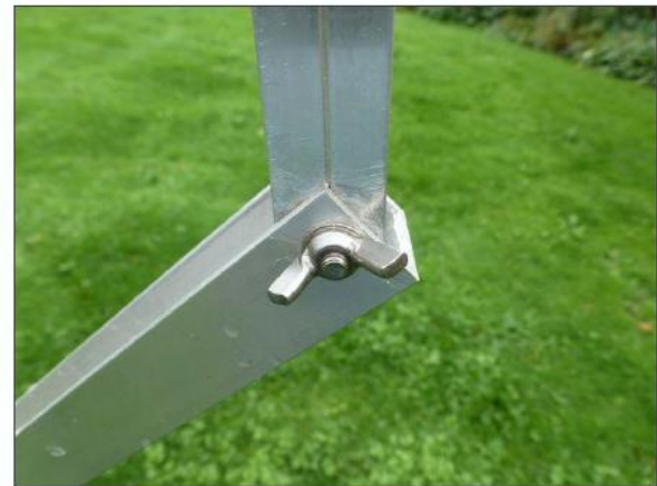
Close up photos of the various joints used to make the Foldable Mag Loop Antenna. The bottom left photo shows the motorised capacitor installed at the base of the loop
