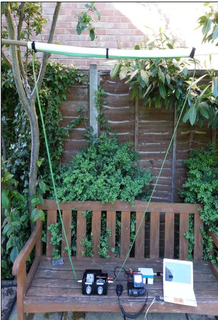
High Power Mag Loop Tuner, Avair 20 SWR meter, Yaesu FT817, external 12v battery box, FoxDelta SWR-Analyser, Acer One netbook
