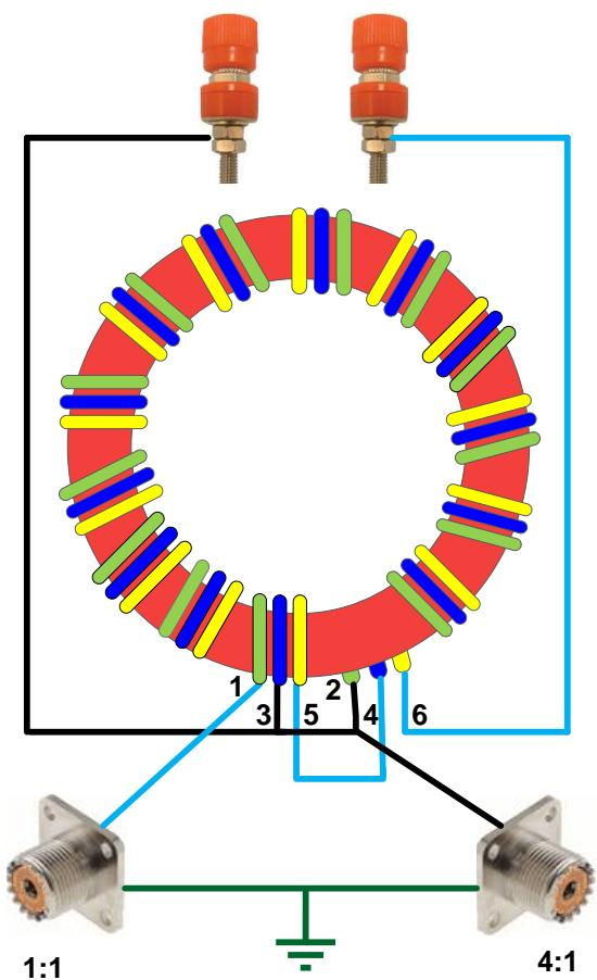
*NOTE:- The tri-filer winding has been shown in three colours to emphasise the way the enamelled copper wires have to be wrapped around the core.*
