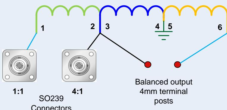
*Note: the windings have been coloured to assist in identifying these on the toroid*
