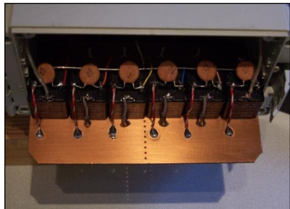
Photo on the LHS shows the copper laminate board pulled forward to provide access to the relay connections. The RG174 coaxes are secured at the rear underside of the board with insulated wire loops. The slack enables the board to be pulled forward.
