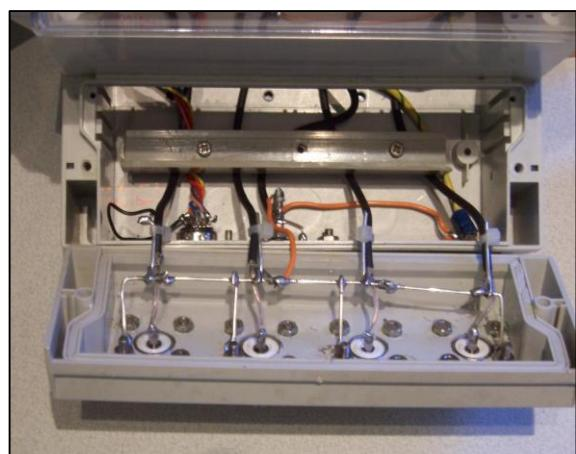
Bottom photo shows the removable front panel with the four SO239 sockets. The silver plated wire support, which is used to secure the braid of the RG174 coax can be seen. The inner is cut slightly longer than the braid so that the braid takes any strain and prevents the inner from breaking off if the cable is accidentally pulled.
