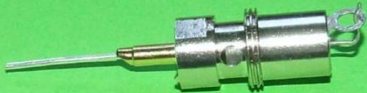
Insert the Type 11A surge arrestor into the nylon tube, which should be a firm fit in the PL259. The end cap should just be visible below the top edge of the connector. The centre pin is soldered to the extension wire.
