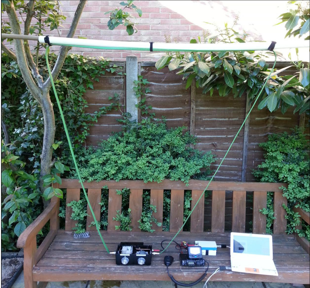
Test set up for the High Power Mag Loop Tuner with thick insulated copper braid (see text)
