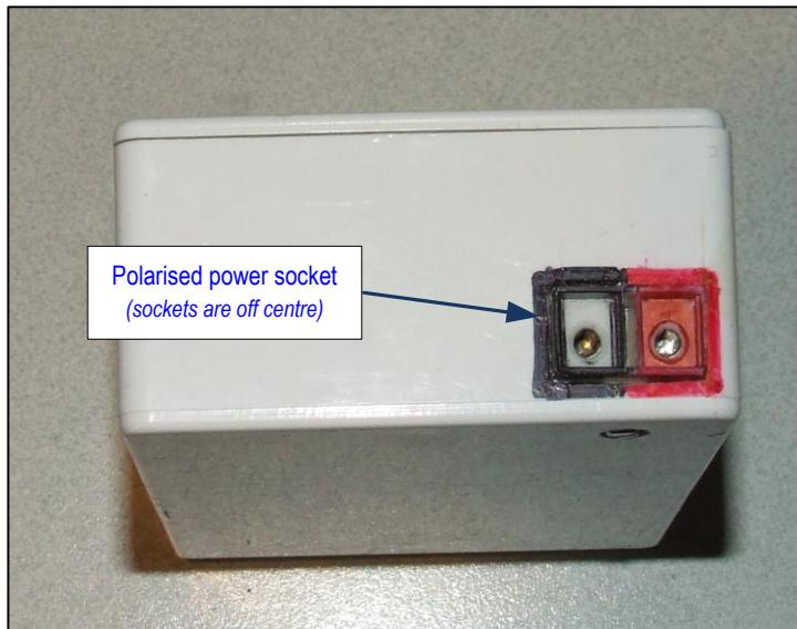
Power connectors are a personal choice but should be polarised so that it is not possible to inadvertently reverse the power to the rig. This is an important point that avoids expensive repairs.
