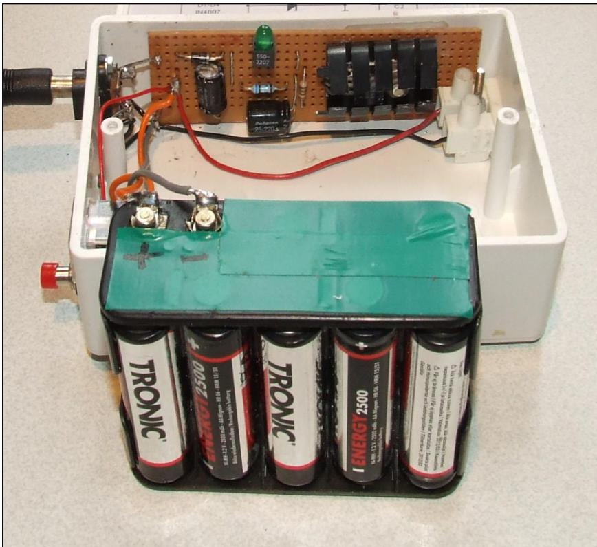
Modify the battery holder by cropping the snap-on connector and adding small solder tags fastened with 8BA bolts through the centre of the original fastenings as shown.
