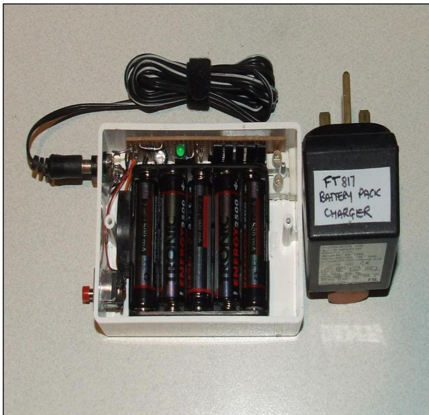
The assembled battery box. The battery holder is held in place by the white output terminal block (top right) and by the black piece of solid rubber on the centre left.
