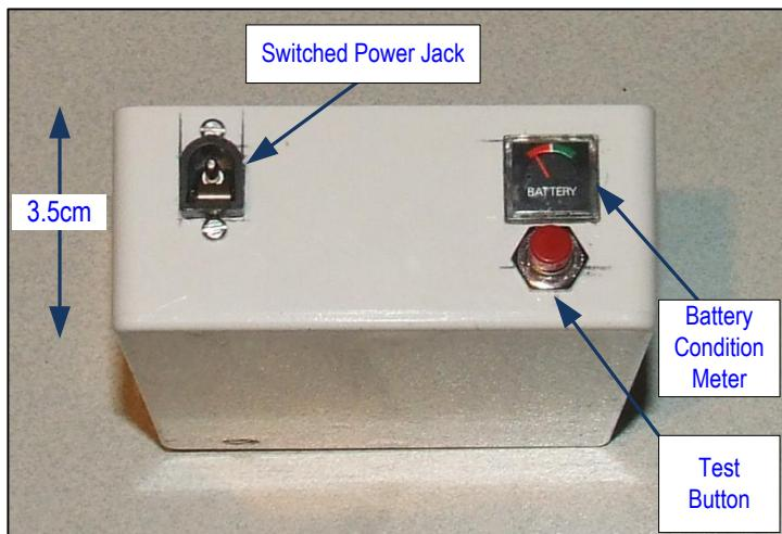
The optional small square battery condition meter from a junk box required a 13.7K resistor for a 15v full-scale deflection (FSD). The centre line indicates 7.5v which is too low for the FT817 to operate. Other meters may require different values for R3
