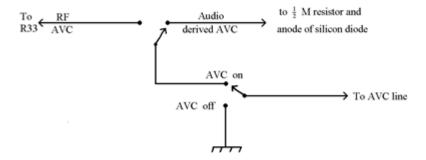
Included in this modification is the re-placing of the BFO "On- off" switch. Remove the toggle switch from the BFO pitch control capacitor (under chassis) and bring the leads up to the hole vacated by the phasing capacitor, where a separate switch is fitted. It is essential on an SSB receiver to be able to leave the BFO tuned to either USB or LSB and be able to switch off the BFO.
