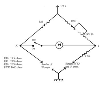
This is a bridge arrangement in which the screens are balanced against the IF valves anode current.
