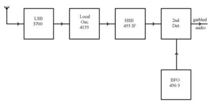
The receiver would not resolve the 80 metre signal
