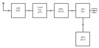
i.e. to receive 80 metre SSB, BFO will be set to 453.7 KHz (depending on the filter)
