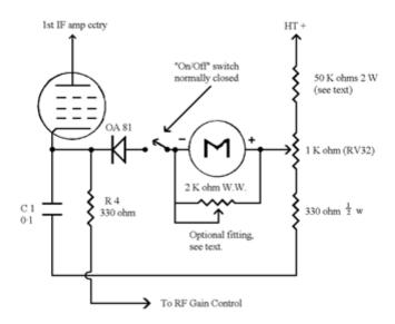
2 Kohm variable resistor (if used) is mounted on rear of meter and is self supporting on heavy wires to meter terminals.
