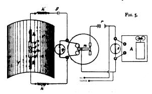
destroyed only for an instance by the tap of the trembler and immediately re-established by the electrical surgings, and therefore the relay tapper and telegraph instrument are again actuated, and so on until the oscillations from the radiator have ceased
