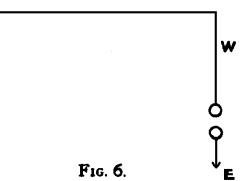
I believe that the exceedingly marked advance made by the adoption of the vertical conductor is due to the fact that the plane of polarization of the rays radiated is vertical, and that therefore they are not absorbed by the surface of the earth, which acts as a receiving conductor placed horizontally. As the maximum effect is obtainable when the conductors of the transmitter and receiver are parallel, this makes it necessary to have a vertical conductor connected to one pole of the coherer.
