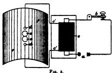
Should it be necessary to direct a beam of rays in one given direction I prefer to use an arrangement similar to a Righi oscillator placed in the focal line of a suitable cylindrical parabolic reflector (f) Fig. 2. The transmitter works as follows: When the key (b) is pressed the current of the battery is allowed to actuate the spark coil (c) which charges the spheres of the Righi oscillator or the vertical wire (w) which discharges through the spark gap.
