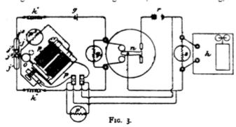
j<sub>1</sub> and j<sub>2</sub> are tightly fitted. They are separated from each other by a small gap, which is partly filled with a mixture of nickel and silver filings. This coherer forms part of a circuit containing the local cell and a sensitive telegraph relay actuating another circuit. which circuit works a trembler, p, decoherer and recording instrument, h.
