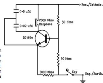
Component values are not critical. Cathode series resistors should be varied to give 4 Volts (approx.). Earpiece has enough output to use as a small speaker for monitoring a CW signal.
