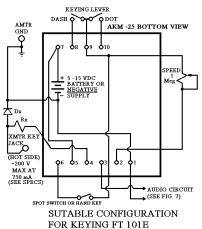
average current. If the key line voltage does not drop to zero with your keyer spot switch closed, Rx should be reduced in value until the key-down voltage does drop to zero.
