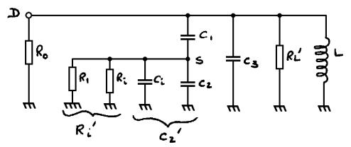
The operating point is set by  $V_{DD}$  and  $R_1$ .  $R_{L'}$  is the transformed value of  $R_L$ , i.e.  $R_{L'} = R_L (n_2/n_1)^2$ .
