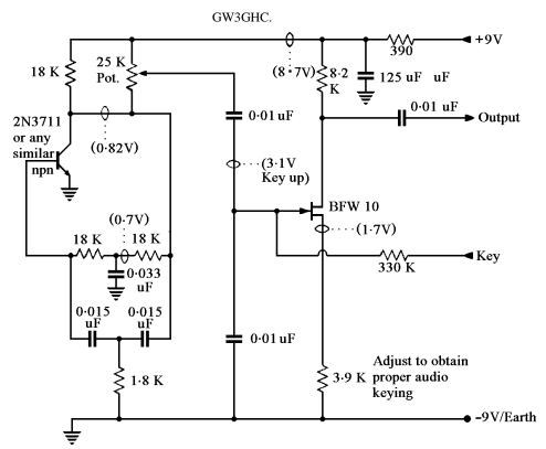
+9V from terminal "CWT" on Carr. Unit (X50-1160-00) Output to terminal "AFU" on AF Unit (X49-1060-00) Key to terminal "Key" on Mixer Unit (X48-1080-00)
