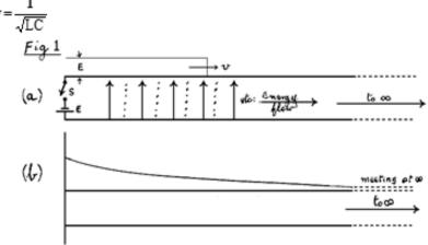
This voltage charges the capacitance of the line producing a current. The current in the wires produces an electromagnetic field between the wires and the voltage an electrostatic field at right angles to the wires. These fields produce an energy flow known as the <u>Poynting</u> Vector in the space between the conductors.
