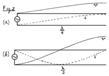
When the line is less than  $\lambda/4$  in length it will look like a capacity (-ye reactance). At  $\lambda/4$  it will look like a series tuned circuit zero reactance and very low resistance, i.e. a short circuit. Between  $\lambda/4$  and  $\lambda/2$  it will look like an inductance (+ye reactance). At  $\lambda/2$  it will look like a parallel tuned circuit, zero reactance and very high resistance, i.e. an open circuit, and so on for each odd and even number of quarter wavelengths.
