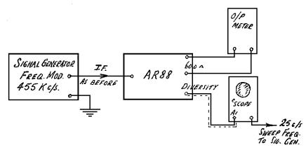
When these connections are made, on the C.R.O. should appear the response curves of the five selectivity positions. Ideally these should be :-
