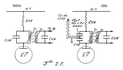
The capacitor C108 is located inside the I.F. transformer
